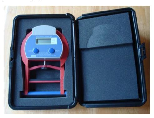
Figure 1. Dynamometer and carrying case
