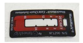
Exhibit 4. Triggered upper threshold temperature monitor
